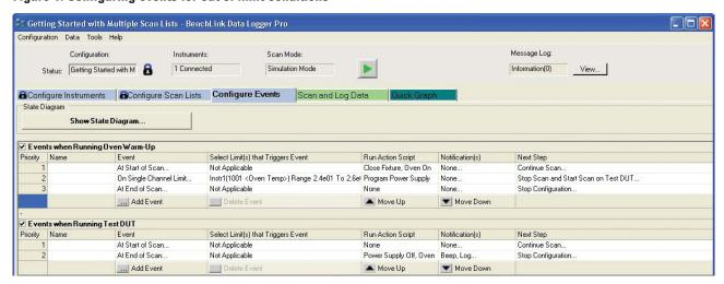
The state diagram feature graphically shows the limits and the order of execution for scan lists, scripts and other notifications. See Figure 2.
